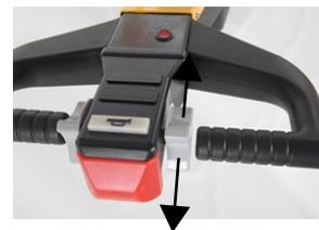
The degree of rotation determines the speed of movement, so the farther you press the wheel in either direction, the faster the E-TUG-HD will travel, up to a maximum speed of ~3.7mph when unloaded or ~2.8 mph when loaded to capacity. Simply by releasing the movement control, the E-TUG-HD will decelerate to a complete stop.
