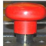
Step 2: Pull the red E-Stop button up to disengage the service brake.
