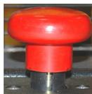
Use The E-Stop as a service brake to secure the E-TUG-HD when parked
