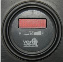
Always check the gauge before using the device; make sure that the battery is charged before using the tugger.
