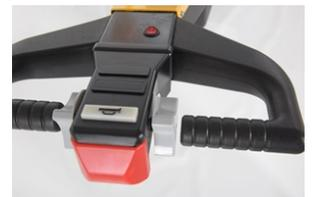
**NOTE:** The E-TUG-HD uses magnetic brakes, which engage when the throttled is turned forward/reverse.
